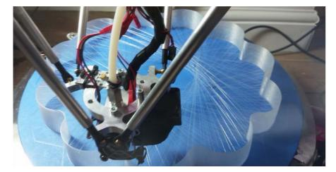
Fig. 29 3D printing in mid-air using silkworm coding, The Cloud Capsules, 2014
