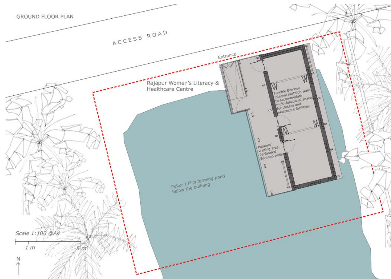
Fig. 44 Post-construction drawing showing the site plan with the building in place
