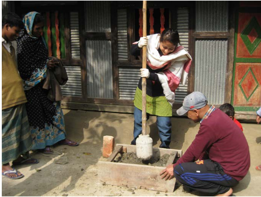
Fig. 45 Earth bricks making skills being shared and demonstrated at the 'Learning Through Making' workshops hosted by the women
