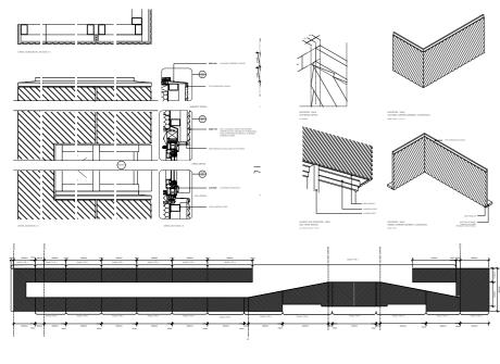
Fig. 16 Camden School for Girls Main Building, construction drawing for pleated glass reinforced concrete (GRC) façade panel design
