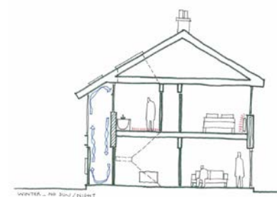
Figs 26-28 Thermo-syphoning sunspace and stairwell, demonstrating connection and isolation from main house to control heat levels. 26: Winter [no sun]; 27: Winter [sun]; 28: Summer [sun/no sun]
